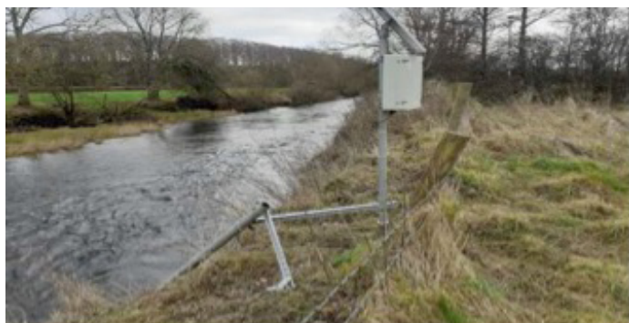
Water Quality Monitoring Station
